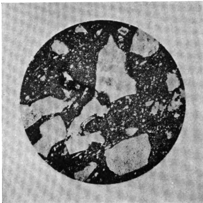
A. PHOTOMICROGRAPH OF A FRAGMENT CONTAINED IN THE ACID VOLCANIC BRECCIA, DAVIDSON COUNTY, N. C. 30 DIAMETERS; ORDINARY LIGHT; SHOWING FRAGMENTARY NATURE OF COMPONENTS.
